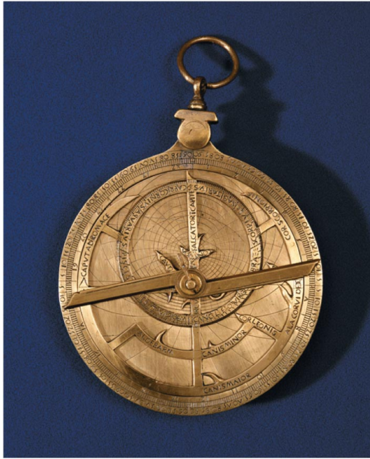
a The faceplate of an astrolabe. Many astrolabes had sighting sticks on the back for measuring positions of bright stars.
